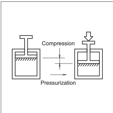
Hydraulic fluid has a small compressibility compared to air but its volume will be reduced by 1% on application of a pressure of 20 MPa {200 kgf/cm<sup>2</sup>}. For this reason, sudden switching of a solenoid valve may cause a shock.
