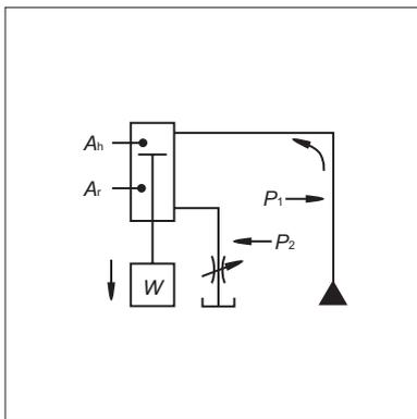
Use of a meter-out throttle as shown in the figure to the left increases the pressure. Especially when the cylinder is directed downward and there is a hanging load however, abnormal pressure at the rod side may occur.
