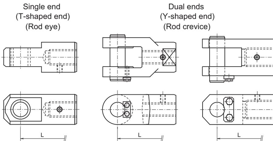
Figure: Example of end bracket
