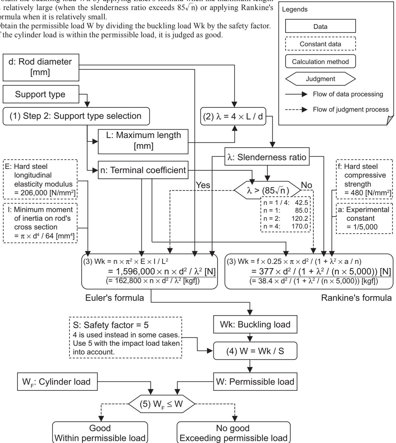
Figure: Flow of buckling calculation
